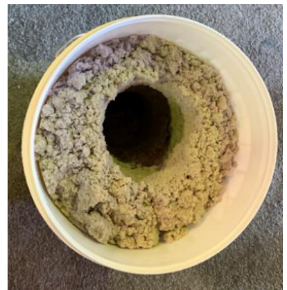
Hole Holding Test – Non-Sagging Epoxy
