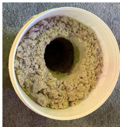
Hole Holding Test – Non-Sagging Epoxy
